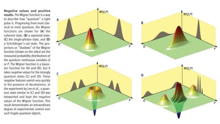
(see the figure, panel A). For a squeezed state, the peak is still Gaussian but now has two-fold symmetry. One variance, say along P, is smaller than the vacuum noise, while the other one is larger (see the figure, panel B). For all optics experiments done during the last century, W(Q, P) was some kind of Gaussian and therefore looked like a "real" (positive) probability distribution.
