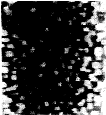
Fig. 6. AFM image of GaSb grown on GaAs:Si using TIPGa and tDMASb at 480°C, average height 6 nm.
