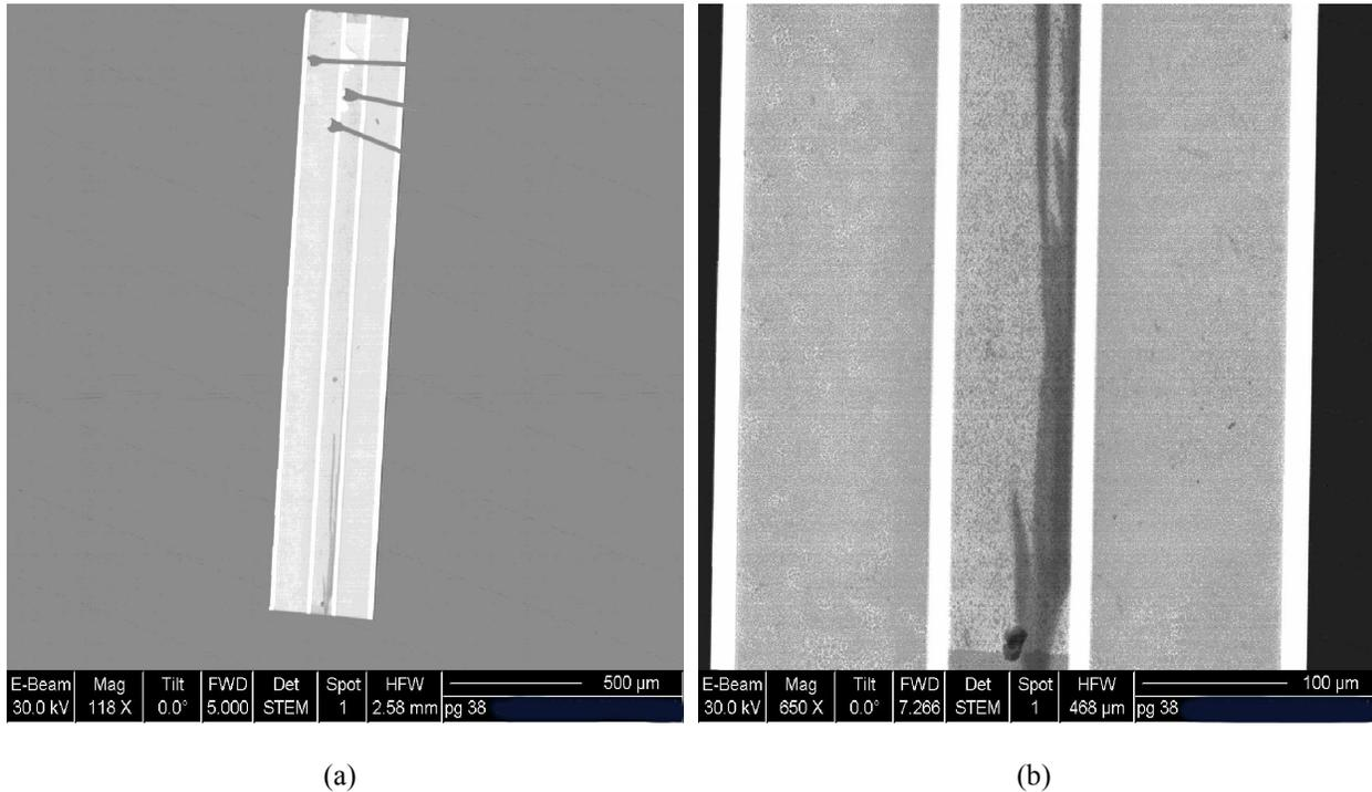
**Figure 2.** EBIC images from Sample A. EBIC images showing the whole chip (a) and front facet area (b) of Sample A.
