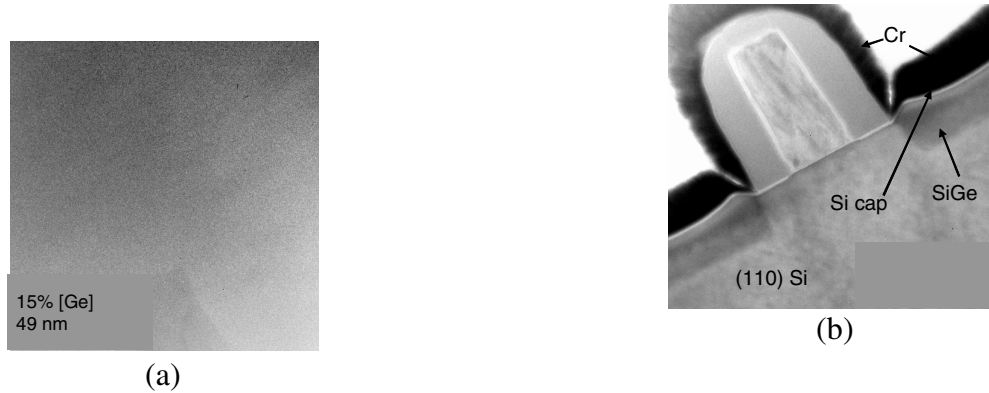
Figure 4 (a): PTEM image of a blanket SiGe film on a 110 Si substrate; (b): XTEM image of a pFET structure with embedded SiGe S/D on a HOT substrate.
