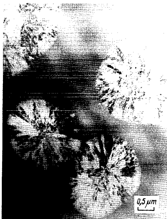
FIGURE 1 Isothermal annealing of Si irradiated by nitrogen ions to a dose of 6 \times 10^{17} \text{ ions} \cdot \text{cm}^{-2} , T_{\text{ann}} = 1100^\circ\text{C} , \Delta t = 5 \text{ min} .
