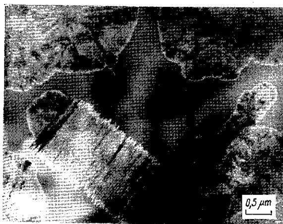
FIGURE 2 Linear dendrite \alpha\text{-Si}_3\text{N}_4 in Si irradiated by nitrogen ions to a dose of 6 \times 10^{17} \text{ ions} \cdot \text{cm}^{-2} , T_{\text{ann}} = 1100^\circ\text{C} , \Delta t = 15 \text{ min} .
