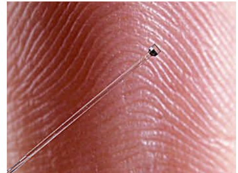
Figure 2 : Miniature FOP-MIV pressure sensor
