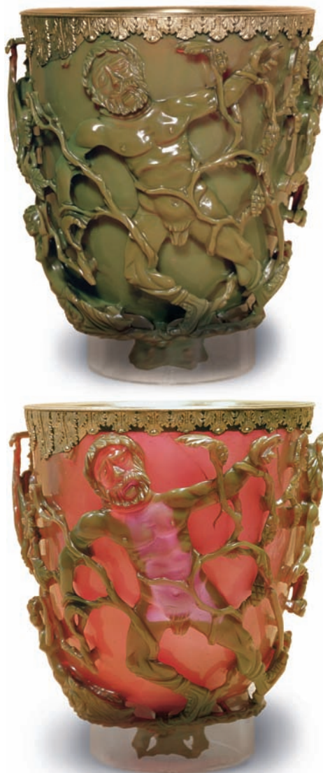
LYCURGUS CUP, a Roman goblet dating from the fourth century A.D., changes color because of the plasmonic excitation of metallic particles within the glass matrix. When a light source is placed inside the normally greenish goblet, it looks red.
