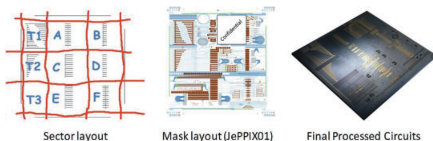
Figure 4 (online color at: www.lpr-journal.org ) Example of a Multi-Project Wafer (MPW) realised in the JePPIX01 process. The wafer is subdivided in 9 sectors, three for test structures and 6 for user designs. The picture in the middle is an example of a mask layout, and at the right is a photograph of the realised wafer.
