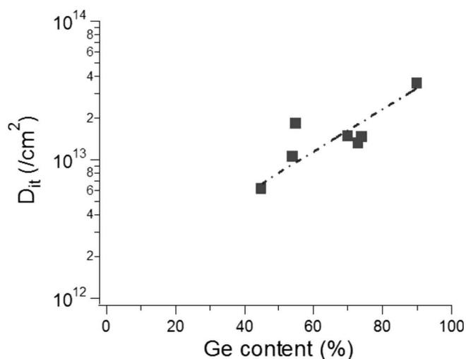
**Figure 10.** Density of interface trap  $D_{it}$  extracted for the different SGOI substrates from the subthreshold slope in weak inversion.
