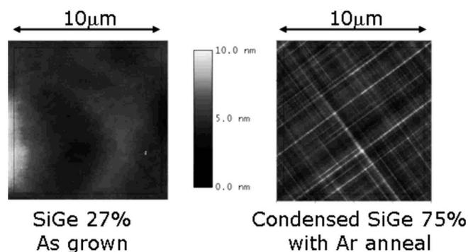
**Figure 3.** AFM image of SGOI substrates before and after the condensation process, showing the appearance of a crosshatch pattern due to the relaxation of the layer.
