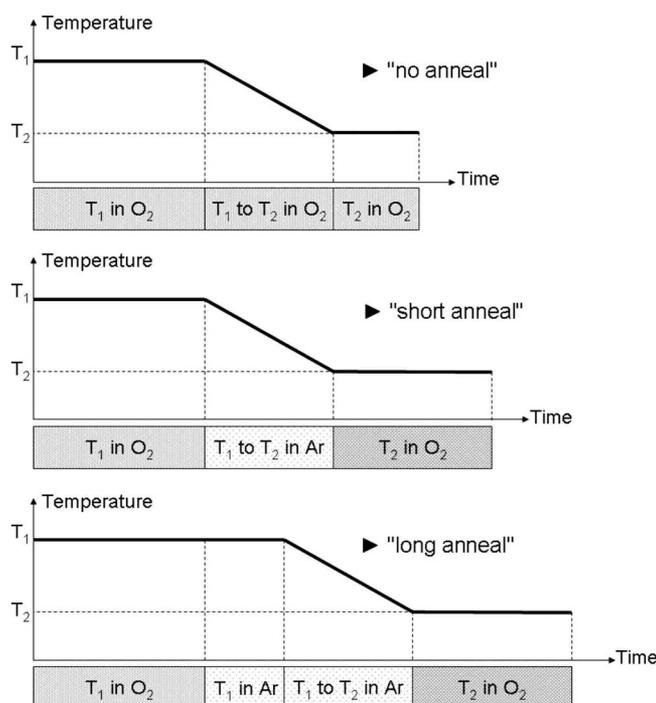
**Figure 1.** Schematic representation of temperature profile and ambient atmosphere in the furnace for the different types of dry oxidation and Ar anneals.
