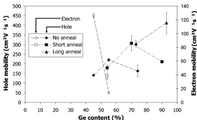
**Figure 9.** Hole and electron low field mobility of SGOI substrates as a function of the Ge content and as a function of the type of anneal used in addition to the condensation.
