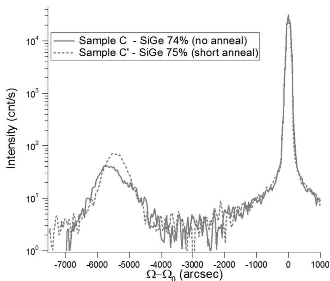
**Figure 5.** High-resolution XRD symmetrical scan around the (004) diffraction peak showing the improvement of the crystalline quality of the SGOI films with 75% Ge atomic fraction when an Ar anneal is used during the condensation process. (The diffraction peak on the left originates from the SiGe film, whereas the right peak is the diffraction peak from the Si substrate.)
