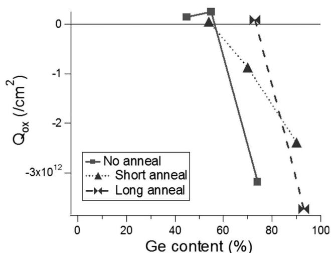
**Figure 8.** Density of fixed oxide charge ( $Q_{ox}$ ) in the BOX as a function of the Ge content in the SGOI and as a function of the type of anneal used in addition to the condensation.
