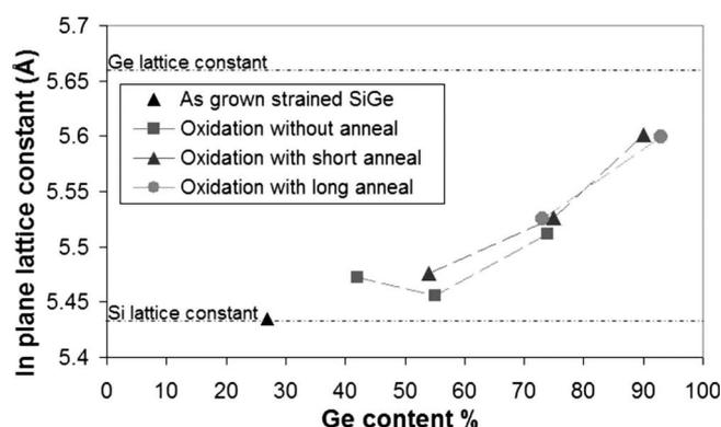
**Figure 6.** Evolution of the in-plane lattice constant of SGOI substrates as a function of their Ge content and as a function of the type of anneal used in addition to condensation.
