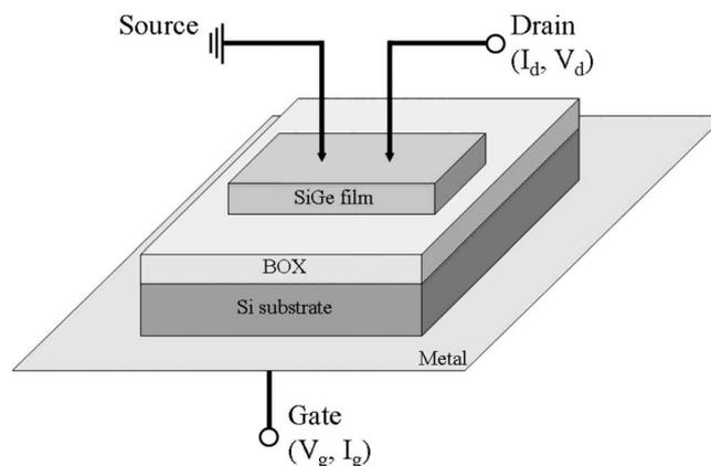
**Figure 2.** Schematic representation of the pseudo-MOSFET measurement.
