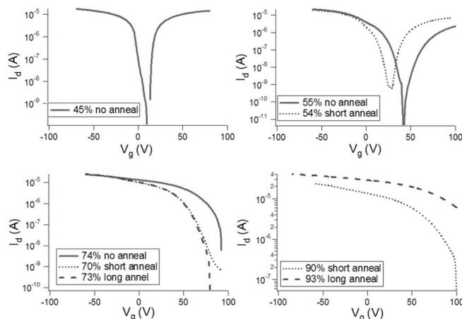
**Figure 7.**  $I_d(V_g)$  characteristics of SGOI substrates measured by the pseudo-MOSFET technique. For the different Ge contents, comparison is made between the different types of Ar anneal.
