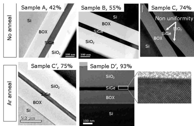
**Figure 4.** Cross-sectional TEM images of the different SGOIs with increasing Ge content. Comparison of sample C and C' clearly demonstrate the beneficial effect of the Ar anneal on layer uniformity.
