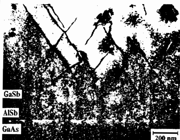
Fig. 4. Cross-sectional bright field micrograph shows the blocking effect of an AlSb buffer to the threading dislocations.
