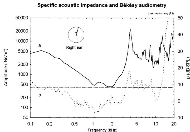
Fig. 7: Comparison between (a) the specific acoustic impedance and (b) hearing thresholds for a subject with a hearing loss of 10-15 dB for 3-10 kHz
