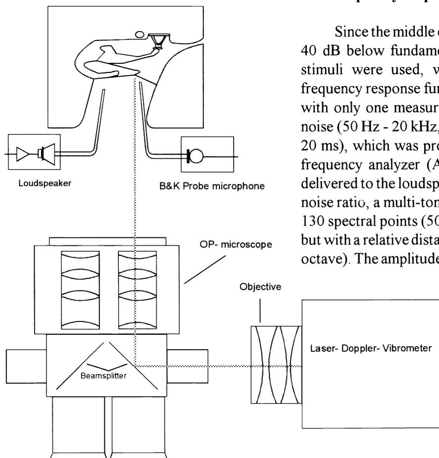
Fig. 2. Schematic diagram of the measurement system for the tympanic membrane.
