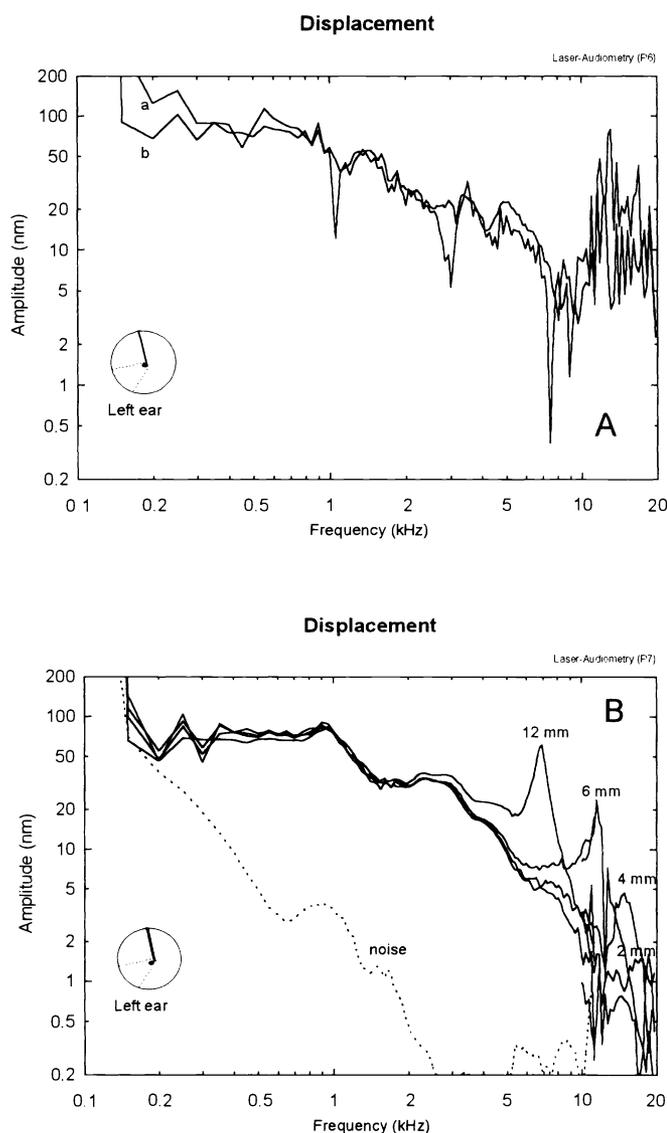
Fig. 5. A: Comparison of amplitude responses of the umbo measured 24 hours apart (b: after 24 hours).
