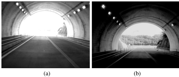
Fig. 16 Comparison of images taken by conversional image sensor (a) and wide dynamic range image sensor (b).
