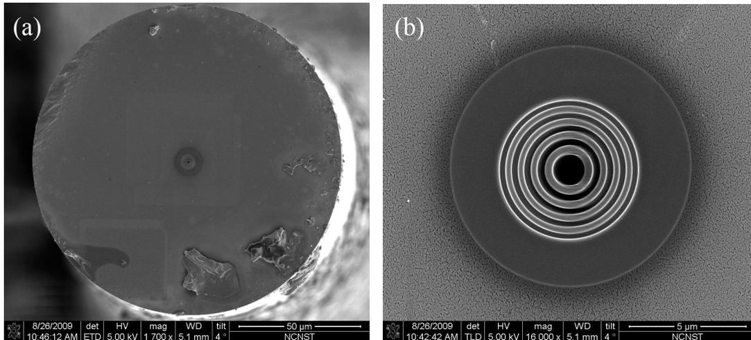
Fig.4 SEM image of the optical fiber tweezers with FZP on the fiber end face. (a) full view of fiber end face with FZP structure, (b) enlarged view of the FZP structure.
