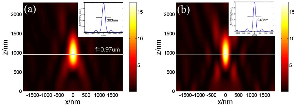
Fig.2 the transverse electric field distribution in (a) XZ plane and (b) YZ plane, the insets are the field distribution along the line in the corresponding plane.
