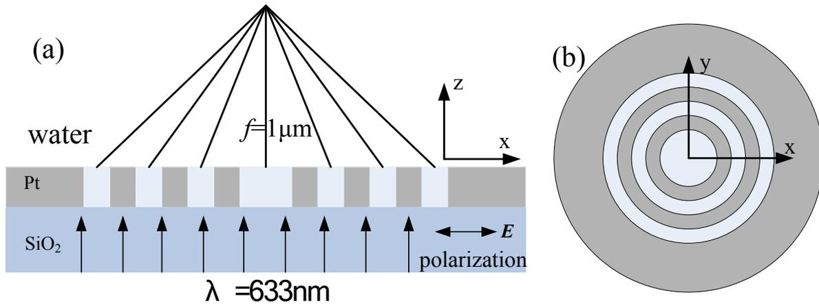
Fig.1 FZP structure diagram. (a) cross section views in xz plane, (b) top-down views
