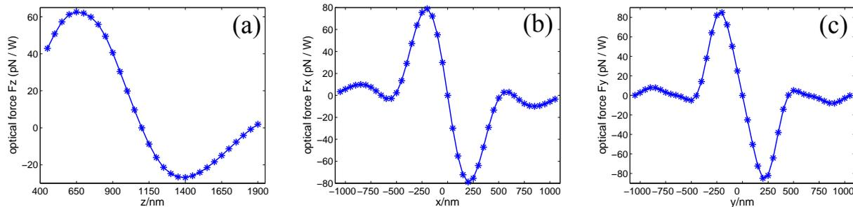
Fig.3. calculation results of the optical force exerted on a 500 nm diameter sphere in the water (a)  $F_z$  along the symmetric axis in different height, (b)  $F_x$  along the  $x$  axis, (c)  $F_y$  along the  $y$  axis in the horizontal plane through  $z$  axial equilibrium point shown in (a)
