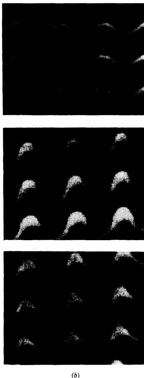
Figure 4. The distortion of a groove profile as the exposure is increased. (a) Diagrammatic representation of the effect on the gradient of refractive index. (b) Scanning electron micrographs of moth eyes of different depths.
