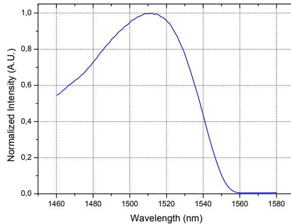
Fig. 2. Experimental wavelength response of the MMI refractometer using No-Core fiber.
