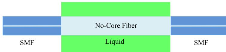
Fig. 1. Schematic of the MMI refractometer.
