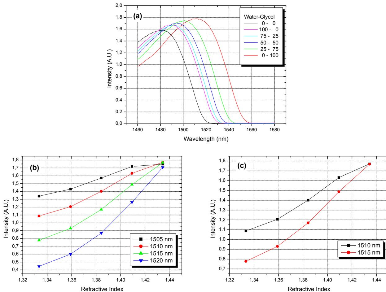
Fig. 3. (a) Wavelength response of the MMI refractometer for different refractive index liquids, (b) Transmitted intensity as a function of different refractive index liquids for specific operating wavelengths, and (c) MMI refractometer response at 1510 and 1515 nm.
