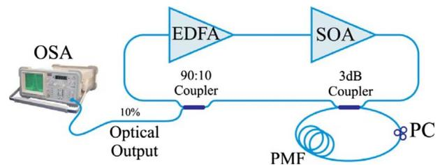
**Fig. 3** The experimental setup; EDFA—erbium-doped fiber amplifier; SOA—semiconductor optical amplifier; PC—polarization controller; PMF—polarization maintaining fiber.
