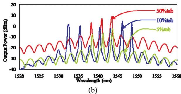
Fig. 4 Result of a multisoliton band with center wavelength at 1.54  $\mu\text{m}$ , where (a) is single output and (b) is tunable output.
