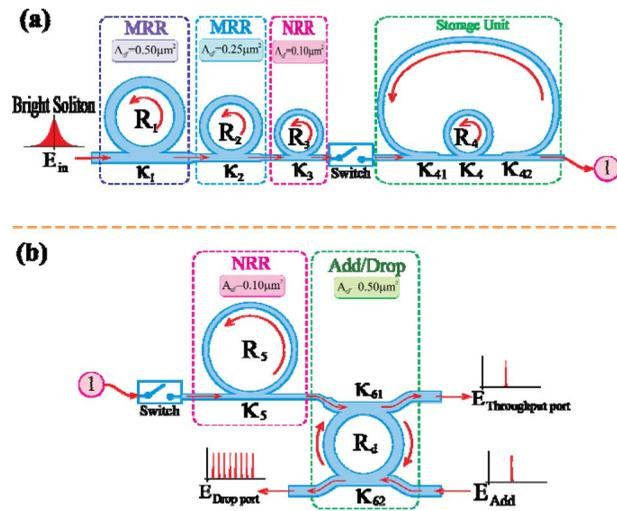
**Fig. 1** A broadband source generation system; (a) a storage unit; (b) a soliton band selector, where  $R_s$  are ring radii,  $\kappa_s$  are coupling coefficients,  $\kappa_{41}$ ,  $\kappa_{42}$  are coupling losses, and  $\kappa_{61}$  and  $\kappa_{62}$  are the add/drop coupling coefficients.
