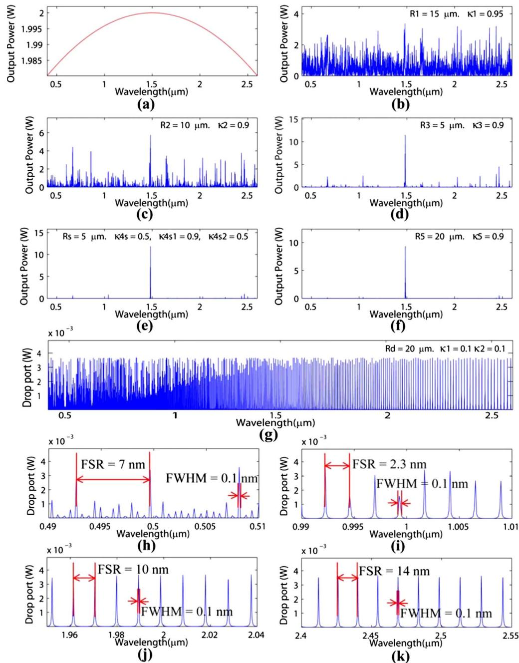
**Fig. 2** A soliton band with center wavelength at  $1.99 \mu\text{m}$ ; (a) input soliton, (b) ring  $R_1$ , (c) ring  $R_2$ , (d) ring  $R_3$ , (e) storage ring, ( $R_s$ ), (f) ring  $R_5$ , and (g), (h), (i), (j), and (k) drop port signals.
