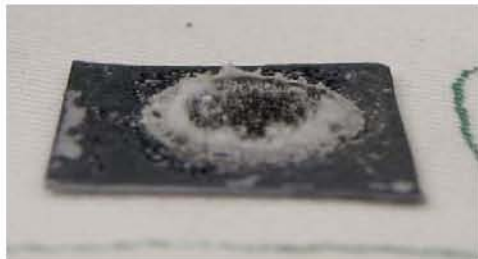
Figure 4 Sample oxidized with 2.4M NaClO 4 in methanol showing migration of salt out of the pores.
