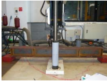
Fig. 3 Hydraulic press system for loading
