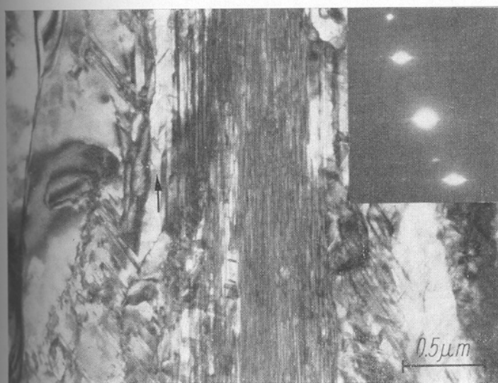
Fig. 1. Structure of silicon crystals in the radial grain area (the arrows indicate the growth directions). a) \langle 200 \rangle growth direction, b) \langle 211 \rangle growth direction
