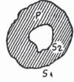
FIG. 2. The superconducting ring P is a multiply connected region. The currents flow only at the surfaces S_1 and S_2 . (From Byers and Yang, reference 6.)
