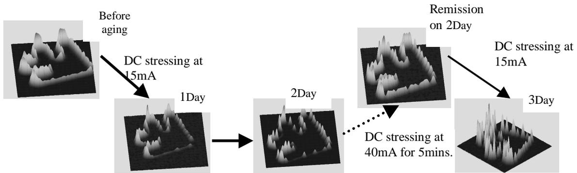
**Figure 9.** Light coalescence as a function of time under DC stressing with breakdown current at 15mA till the 2<sup>nd</sup> day. After 5min of high current DC stressing at 40mA, causes remission phenomenon. Coalescence behavior reappears when re-stressed at 15mA for 1day
