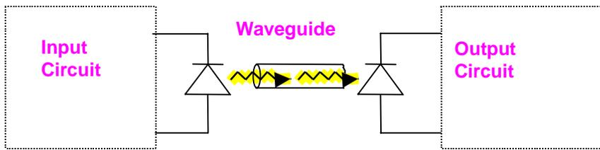
**Figure 1** Concept of on-chip optical inter-connects with Si emitter, waveguide, receiver.
