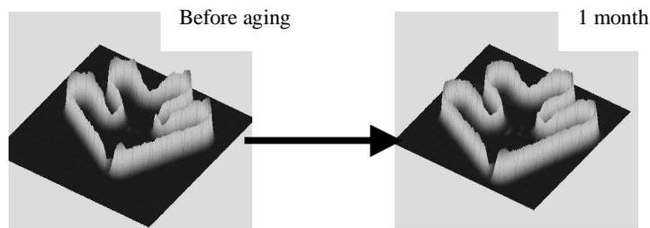
**Reliability** **Figure 7** Spatial variation of emission from p-n junction subjected to DC stressing with breakdown current at 46mA. No light coalescence observed.
