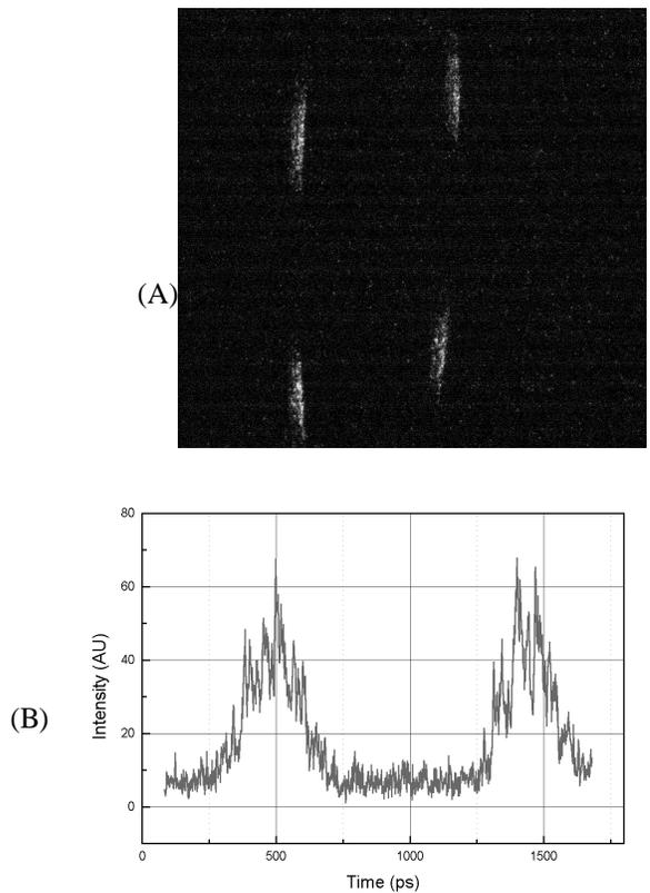
**Figure 6** a) Streak Camera (C5680) image of light emission from the CW excitation. b) Intensity of light emission vs time plot.
