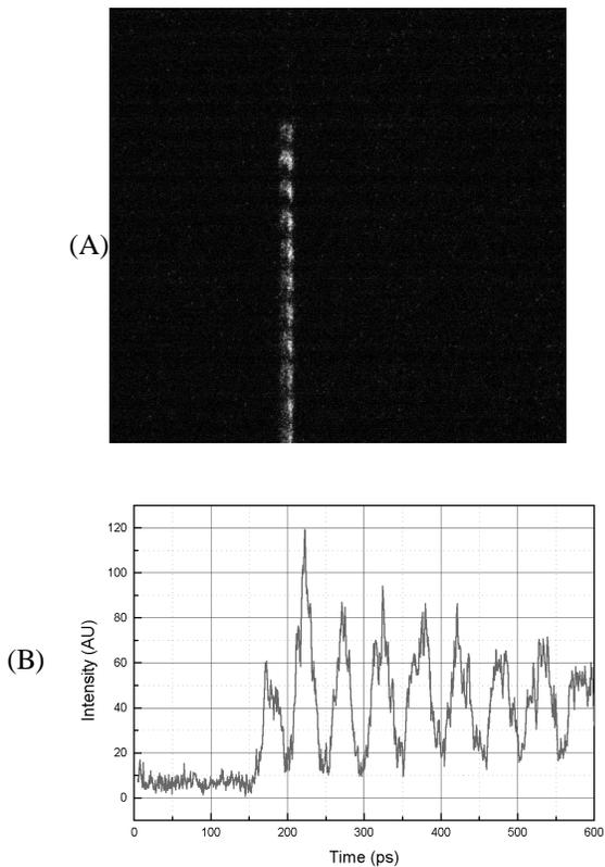
**Figure 5** a) Streak Camera (C5680) image of light emission from the pulsed excitation shows the device response in the pico-second range. b) Intensity of light emission vs time plot.
