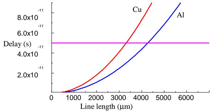
**Figure 4** Line delay compared for Aluminum, Copper and optical interconnect.
