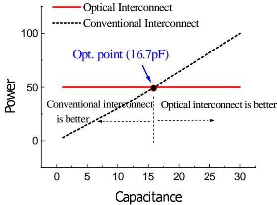
**Figure 3** Power comparison between two systems in terms of line capacitance.
