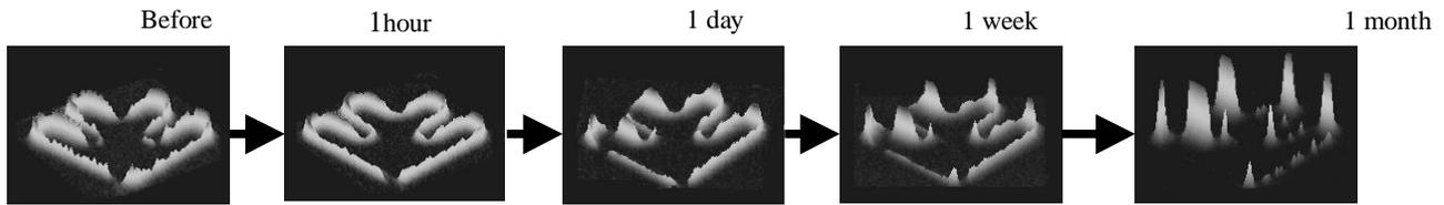
Figure 8. Light coalescence as a function of time under DC stressing with breakdown current at 24mA.
