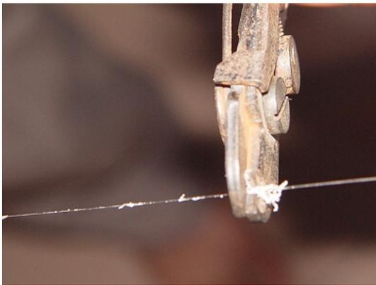
Fig.1 Decoating the polymer of naked optical fiber
