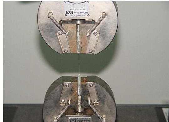
Fig.3 Tensile test in Instron 5567
