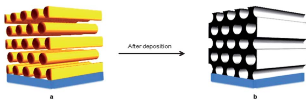
Fig. 7 A schematic representation of (a) the shear aligned H_1 templating phase and (b) the corresponding aligned H_1 -ePt film produced by electrodeposition.
