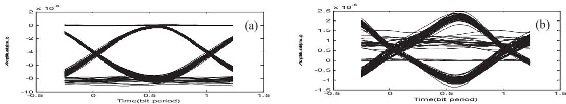
Fig.10 Eye diagram after demodulation in different transmission distance at base station(a)30km (b)40km
