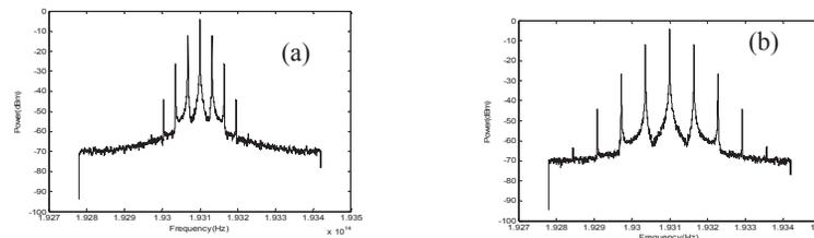
Fig.3 The modulated signal after modulating by a MZM with different modulated signal (a) 32GHz (b) 64GHz
