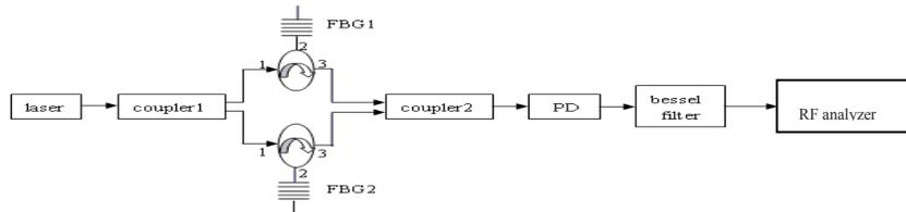
Fig.8. The structure of the MPG based on FBG
