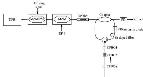
Fig.1 The structure of the tunable MPF
