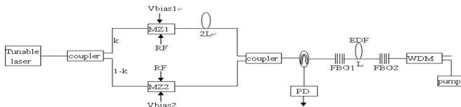
Fig.5 The structure of the flat MPF
