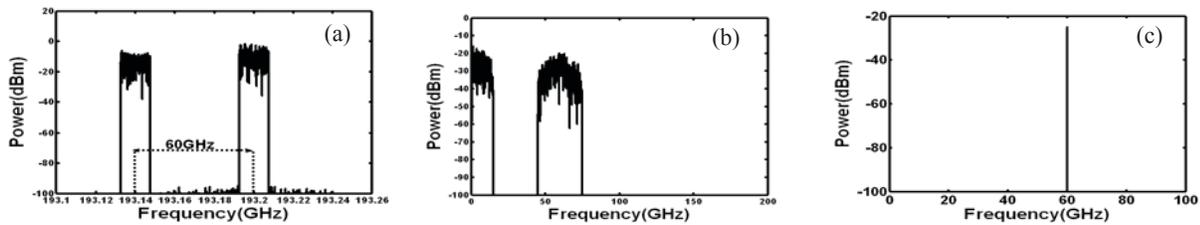
Fig.9 The spectrum of MPG (a) Heterodyne light before PD (b) Output of PD (c) 60GHz millimeter wave after filtering
