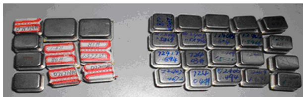
Fig. 5 Vacuum packaged samples by resistance welding
