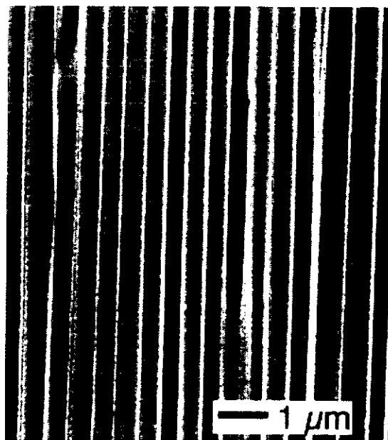
Fig. 24. Cross-section of the self-organized pore array in anodic alumina obtained using a two-step anodization process. Reprinted with permission from [49]. A. P. Li et al., Electrochem. Sol.-St. Lett. 3, 131 (2000). © 2000. ECS.
