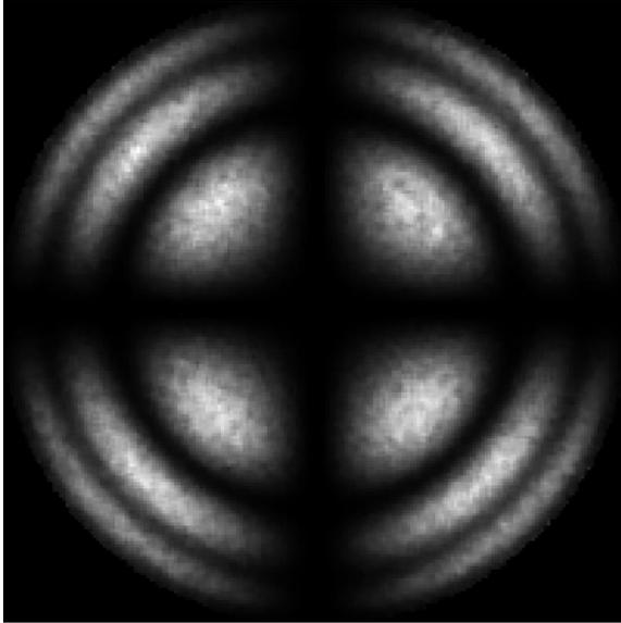
**Figure 11 Polarization interference of ideal c-plate**
