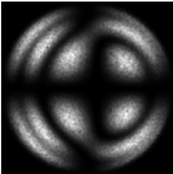
**Figure 12 Polarization interference of non-ideal c-plate**
