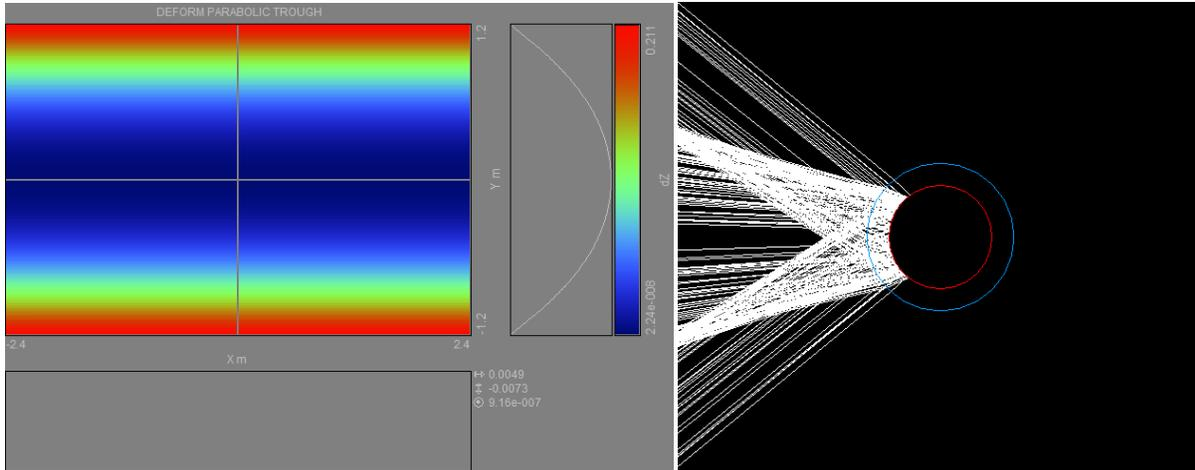
**Figure 17 Deformed parabolic trough and energy distribution**
