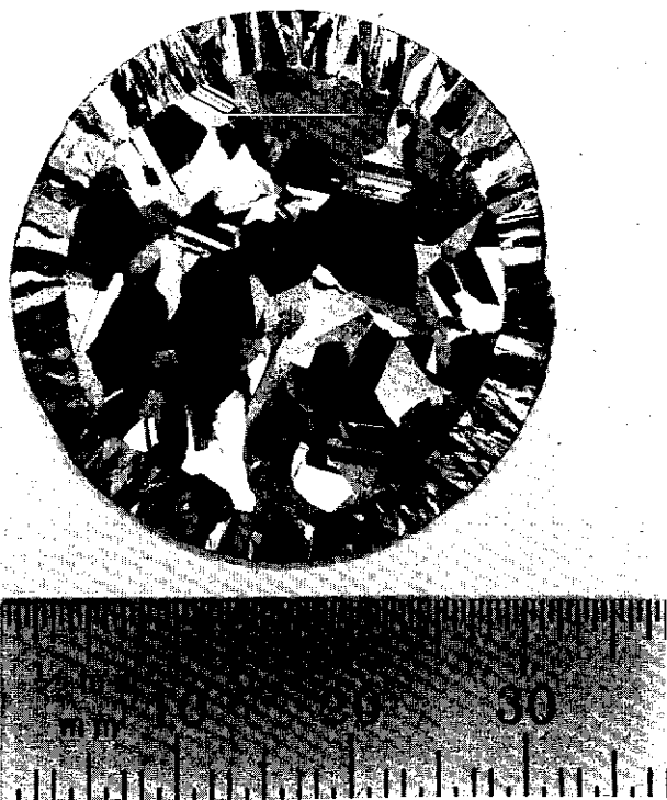
Fig. 2. Etched cross section of silicon directionally solidified in a cold crucible.
