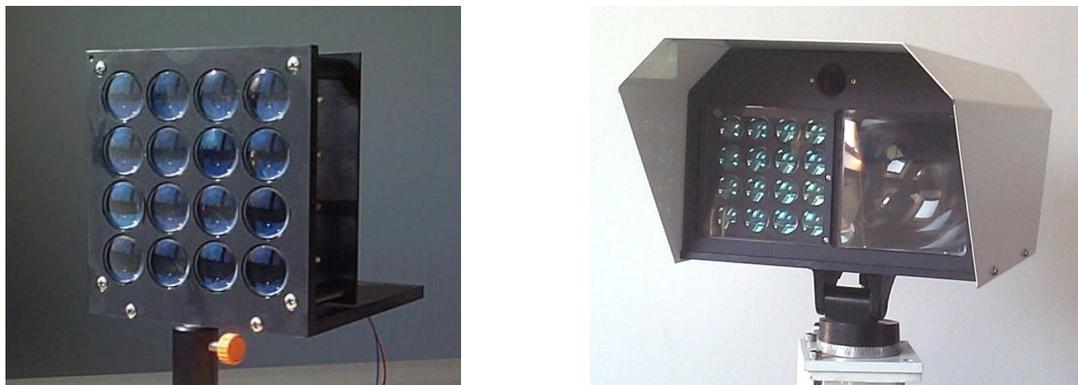
**Figure 11.**  $4 \times 4$  VCSEL beam FSO module in a test version (*left*) and integrated into a complete FSO transceiver device (*right*).
