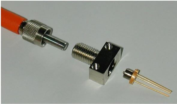
**Figure 15.** Photograph of a VCSEL-SMA fiber receptacle before assembly. The 25  $\mu\text{m}$  diameter VCSEL is mounted onto a TO-56 header with a ball lens cap.
