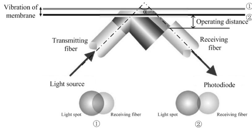
Fig.1 Principle of fiber acoustic sensor
