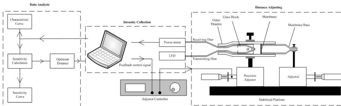
Fig.4 Illustration of packaging system
