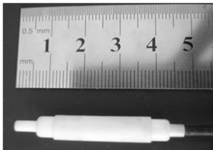
Fig.7 The photo of packaged fiber acoustic sensor
