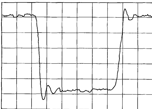
Fig. 3. Typical waveform of the current signal due to electron transport at 300°K. The width of the diode is 500 \mu m , and the applied voltage is 1250 V. The drift velocity obtained from this signal is 9.23 \times 10^6 \text{ cm/sec} . Horizontal Sensitivity 1 ns./division.
