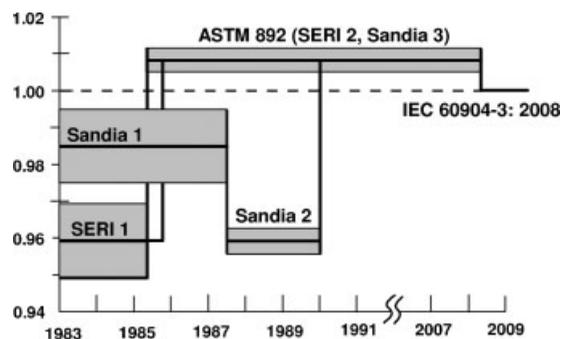
Figure 2. Calibration factor multiplier allowing conversion of past short-circuit current measurements to present standards
