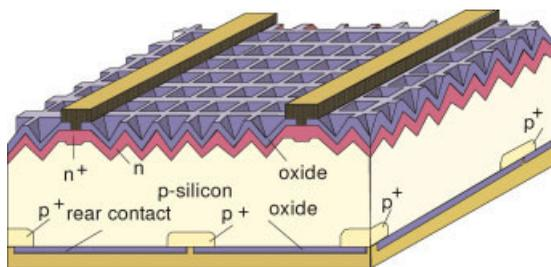
Figure 1. PERC cell
