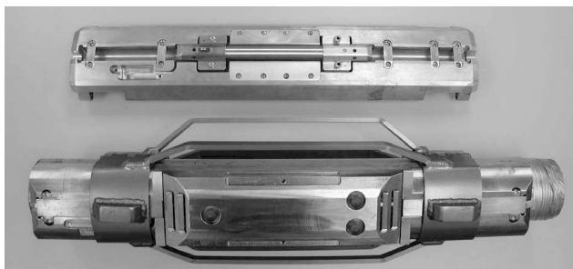
Figure 18. Prototype active seismic clamp (top) and subsequent production-well design (bottom).
