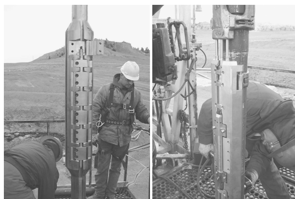
Figure 8. (Left) Final PSM prototype. A threaded mandrel was ultimately chosen for minimizing production-well deployment risk. The optimal mandrel shape was determined to be tubular, concentric to the borehole. (Right) Final ASC prototype, designed to house the 3C fiber-optic accelerometers in a clamp-on device, similar to a cable protector. The design uses a spring-loaded pad to couple the sensor package to the casing, isolating as much as possible the three accelerometers from the clamp, tubing, and the connected fiber-optic cable.
