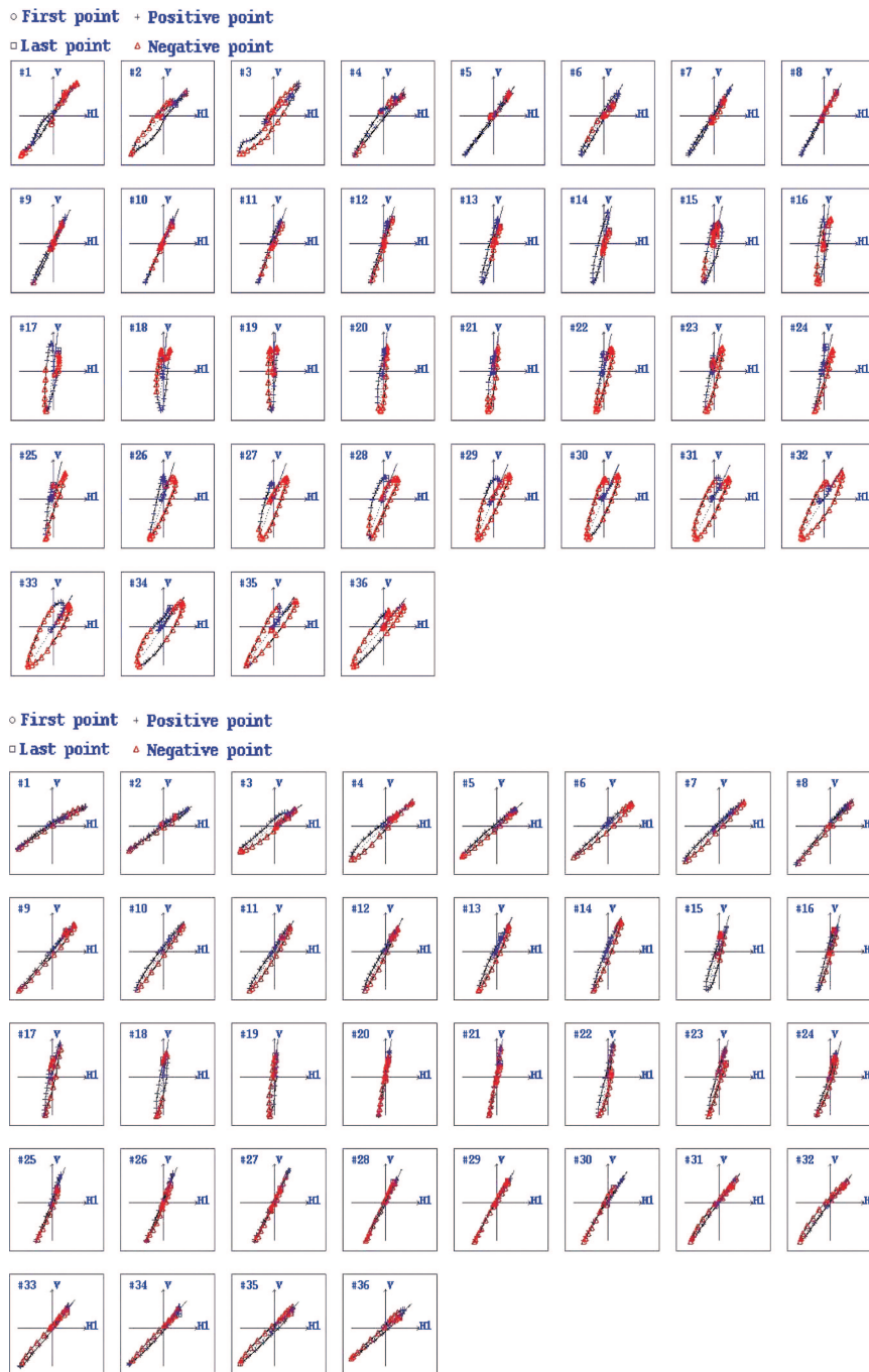
Figure 13. Hodograms from both the ASC (bottom) and PSM (top) show good tracking of the source as it traverses a walkaway line.
