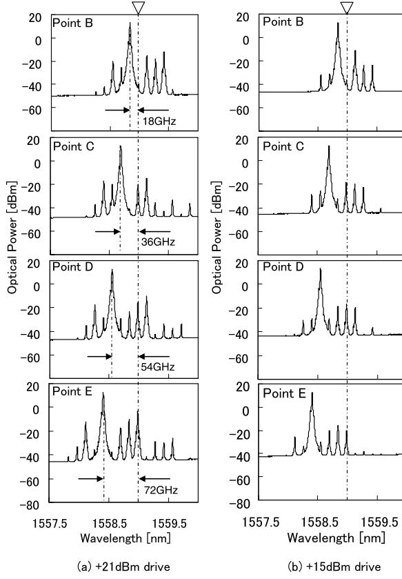
**Fig. 2** Optical spectrum of wavelength converter outputs.
