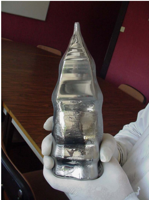
Fig. 1 As grown GaSb:Te crystal Se_127 grown by Cz process
