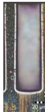
FIGURE 3. Junction staining on a conformally doped 200 \mu\text{m} deep trenches
