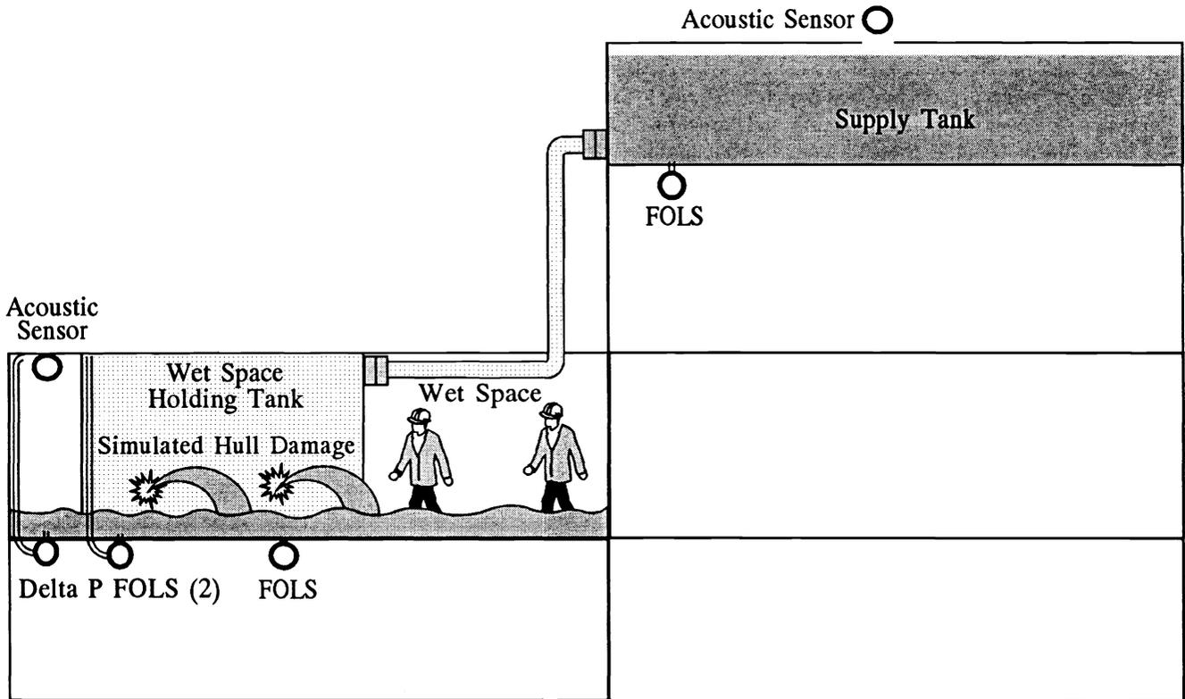
Figure 7 - Differential Pressure Sensor Installed on Ex-USS SHADWELL
