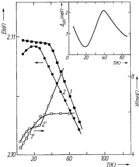
Fig. 4. Energy shift (curves 1 and 2) and broadening (curves 1' and 2') with increasing temperature of PL lines corresponding to (1), (1') emission of a free exciton ( $I_{FES}$ -line) in pure GaSe and (2), (2') of a localized exciton ( $I_{LES}$ -line) in GaSe:Mn crystals. Insert: temperature dependence of  $\Delta_{LES}$ .
