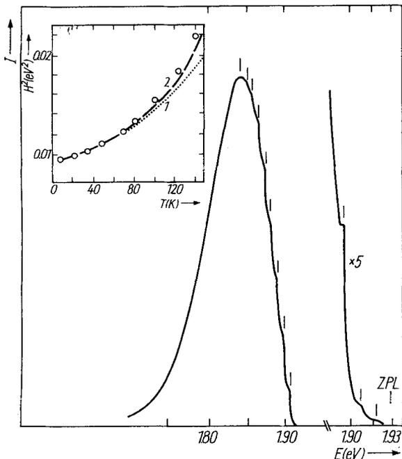
Fig. 2. PL spectrum of the impurity band of GaSe: Mn (0.5 wt%) crystal at  $T = 4.5$  K. Insert: temperature dependence  $H^2(T)$ ; open circles experimental data, (1) according to (1), (2) according to (2).
