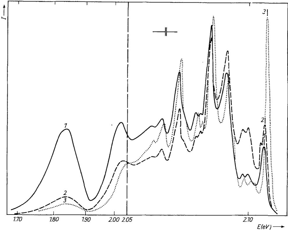
Fig. 1. PL spectrum of GaSe:Mn (0.5 wt%) crystals at  $T = 4.5$  K from different crystal regions
