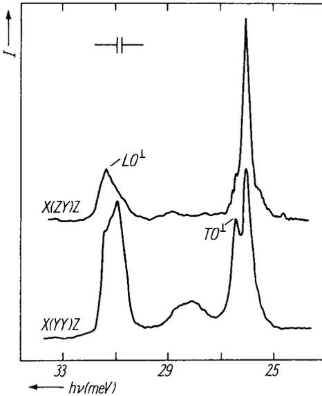
Fig. 3. Polarized Raman scattering spectra of GaSe: Mn(0.5 wt%) crystal at  $T = 300$  K in right-angle geometry ( $z \parallel c$ -axis),  $E_i = 1.92$  eV
