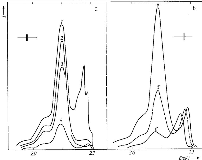
Fig. 5. PL spectra of GaSe(Mn) crystal at (1)  $T = 4.5$  K, (2) 20, (3) 30, (4) 45. (5) 60, and (6) 80 K. Curves 4 to 6 in b) are shown with fivefold magnification
