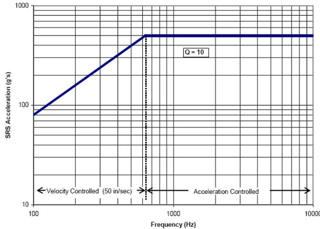
Figure 6: Representative Pyroshock Requirement<sup>[8]</sup>
