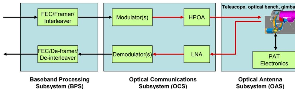
Figure 1: Space Lasercom Terminal Functional Block Diagram
