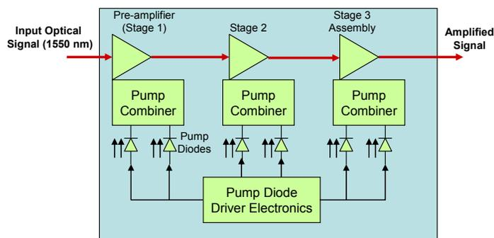
Figure 3: High-Power Optical Amplifier Block Diagram
