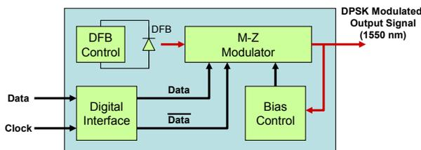
Figure 2: Optical DPSK Modulator Functions
