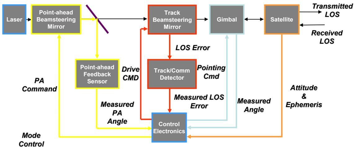
Figure 4: Pointing, Acquisition, and Tracking System Block Diagram
