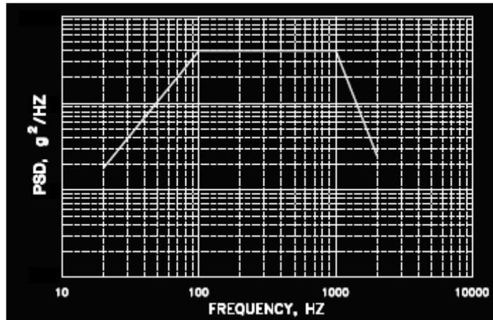
Figure 5: Representative Random Vibration Requirement<sup>[6]</sup>
