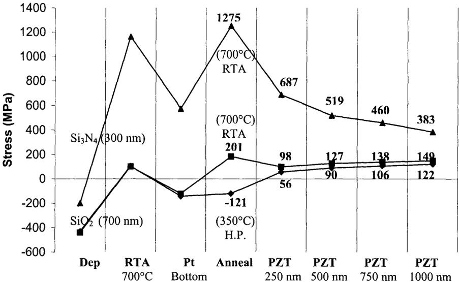
**Fig 1.** Measured stress at different deposition and annealing steps for two SiO<sub>2</sub> and one Si<sub>3</sub>N<sub>4</sub> dielectric test wafers.
