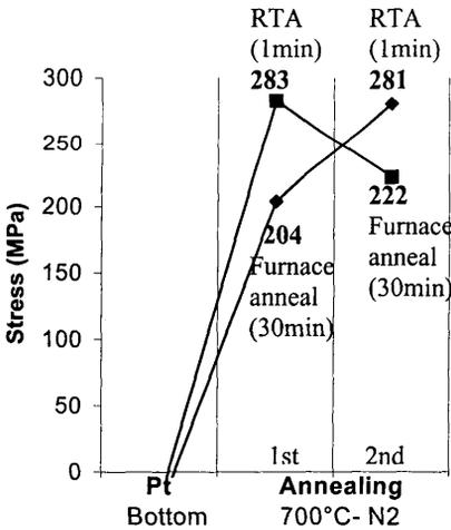
Fig 2. Effect of two separate annealing treatments on platinized oxide substrates.
