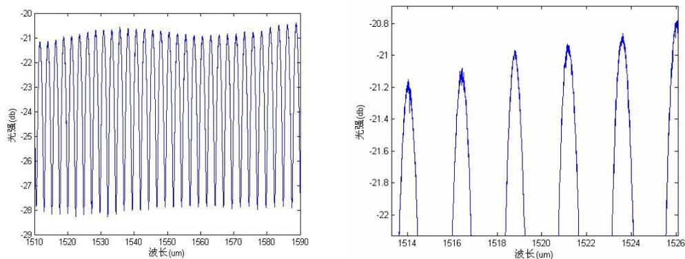
Fig.5 Spectrum before wavelet de-noising
