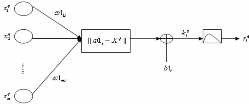
Fig.2 Input and output of hidden layer neuron of RBF network
