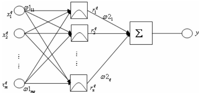
Fig.1 Structure of RBF network
