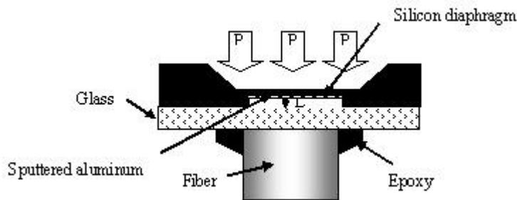
Fig.4 The sketch of optical fiber MEMS pressure sensor
