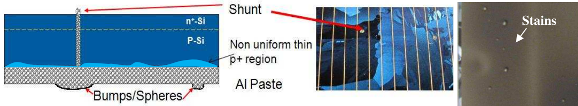
Figure 1. Schematic illustrating various issues involved in good back-contact formation.
