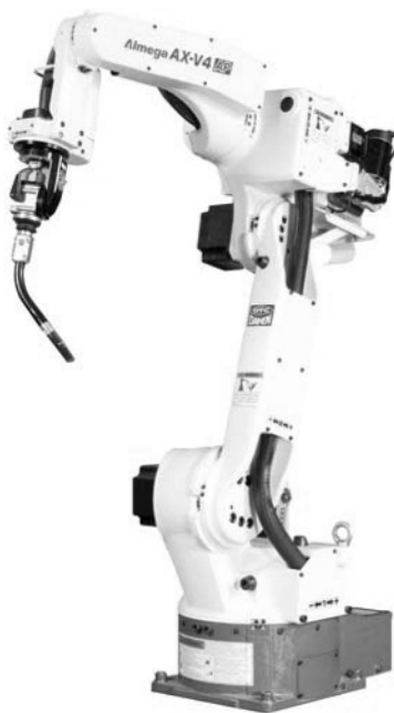
Figure 1.20 Welding robot for car manufactory (courtesy of Rolan-Robotics)
