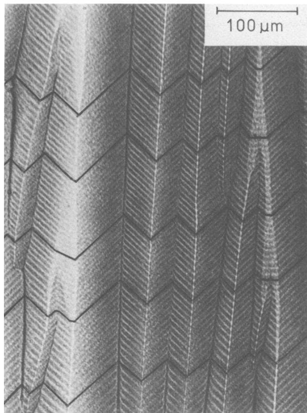
Fig. 6. Micrograph of an Si film recrystallized by zone-melting showing experimental evidence in support of the model presented in Fig. 5. The instantaneous solid-liquid interface was demarked by pulsing the upper strip-heater at 120 Hz. Approximately every twelfth demarcation line is traced in ink to clarify the time evolution of the solidification front. Seam direction is from top to bottom.
