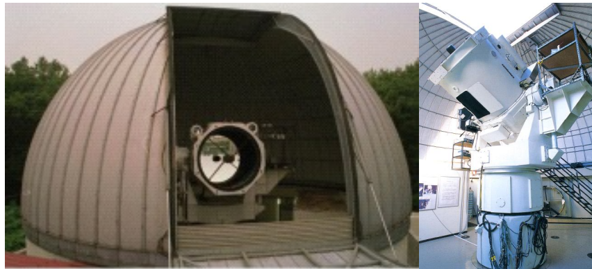
Figure 4 NICT's optical ground station. The diameter of the telescope aperture is 1.5 m.
