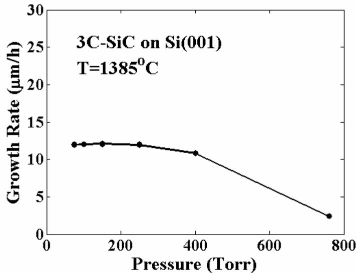
Figure 3. 3C-SiC film growth rate vs. process pressure. Films grown at a speed of 12  $\mu\text{m/h}$ . Process Si/C and Si/Cl ratios of 0.9 and 6.5, respectively. Trend line drawn to aid the eye only.
