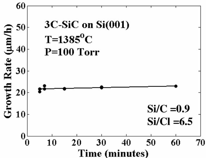
Figure 4. 3C-SiC film growth rate vs. growth time. The films were grown at a rate of 20  $\mu\text{m/h}$ . The growth times were 5, 7, 15, 30 and 45 min. Process Si/C and Si/Cl ratios were 0.9 and 6.5, respectively. Trend line drawn to aid the eye only.
