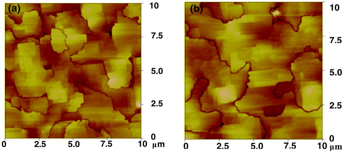
Figure 2. Plan-view AFM micrographs of 3C-SiC films grown for equal time at (a) 20  $\mu\text{m/h}$  and (b) 38  $\mu\text{m/h}$ . Film thicknesses are 2.1  $\mu\text{m}$  and 3.6  $\mu\text{m}$ , respectively. Scan area 10 $\mu\text{m}$  x 10 $\mu\text{m}$ .
