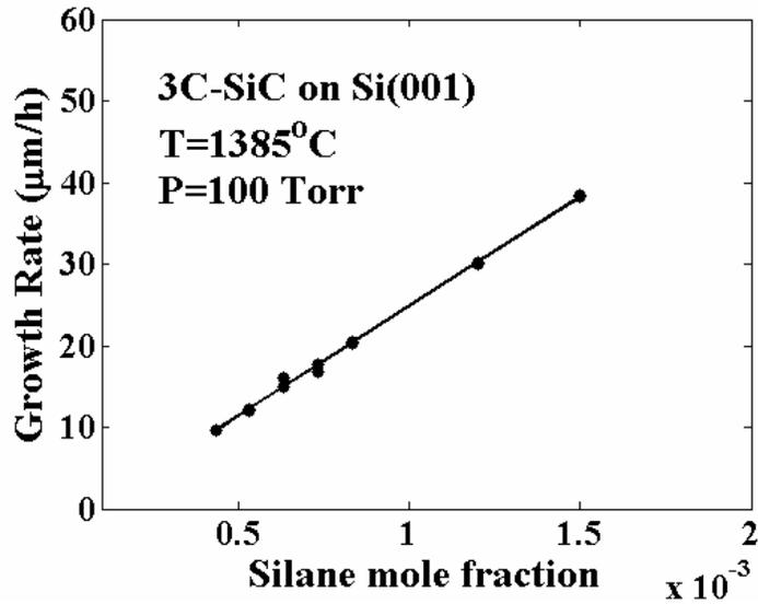
Figure 1. 3C-SiC film growth rate vs.  $\text{SiH}_4$  flow rate. The process Si/C and Si/Cl ratios were 0.9 and 6.5, respectively. The solid trend line is used to aid the eye only.
