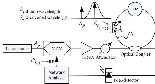
Fig.1 Schematic diagram of a new SOA-based microwave photonic notch filter. MZM: Mach-Zehnder modulator; EDFA: erbium-doped fiber amplifier, SOA: semiconductor optical amplifier, TNOF: tunable narrow-band optical filter
