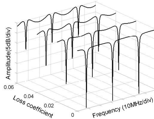
Fig.4 Theoretical overall frequency responses of the filter structure as the function of  $L_1$
