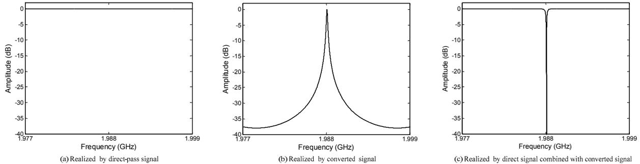
Fig.2 The derivation of the notch filter with flat passband
