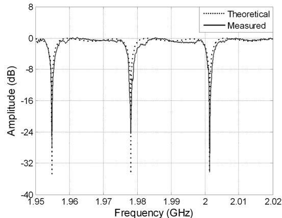
Fig.5 Theoretical and measured frequency responses of SOA-based microwave notch filter with 50:50 coupler
