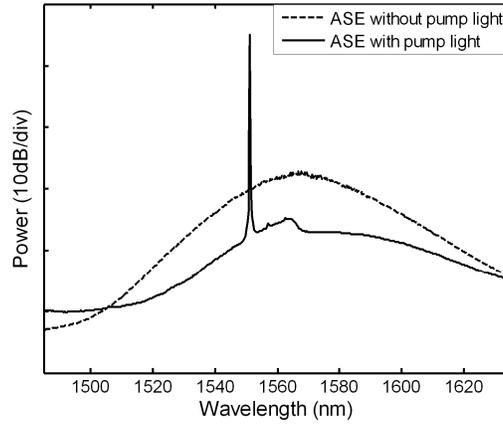
Fig.3 Measured ASE spectrum of the SOA with and without pump light
