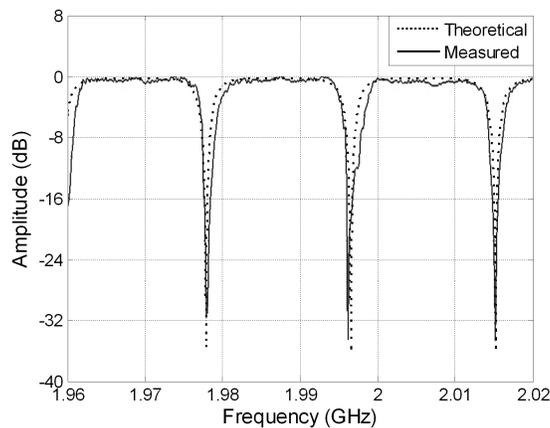
Fig.6 Theoretical and measured frequency responses of SOA-based microwave notch filter with 30:70 coupler
