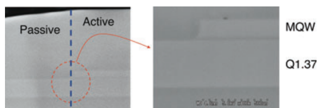
Figure 17 (online color at: www.lpr-journal.org ) SEM image of the active/passive interface in the fabricated PIC.
