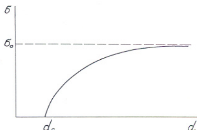
Fig. 15. Dependence of growth interface supersaturation on diameter of whisker (and/or of droplet). \sigma_0 is determined by molar concentration of reaction mixture.
